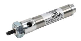
NITRA pneumatic cylinder, non-repairable, 3/4in bore, 1/4in rod diameter, 1-1/2in stroke, double acting, front nose mount.
