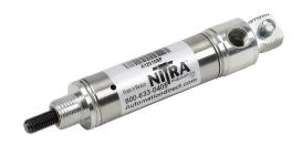
NITRA pneumatic cylinder, non-repairable, 3/4in bore, 1/4in rod diameter, 1in stroke, single acting, rear pivot mount.
