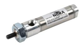
NITRA pneumatic cylinder, non-repairable, 3/4in bore, 1/4in rod diameter, 1in stroke, double acting, front nose mount.
