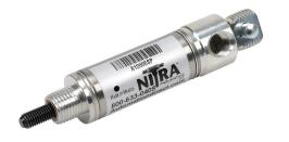
NITRA pneumatic cylinder, non-repairable, 3/4in bore, 1/4in rod diameter, 1/2in stroke, single acting, rear pivot mount.
