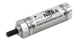
NITRA pneumatic cylinder, non-repairable, 3/4in bore, 1/4in rod diameter, 1/2in stroke, single acting, front nose mount.
