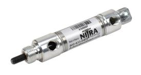
NITRA pneumatic cylinder, non-repairable, 3/4in bore, 1/4in rod diameter, 1/2in stroke, double acting, rear pivot mount.
