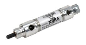
NITRA pneumatic cylinder, non-repairable, 3/4in bore, 1/4in rod diameter, 1/2in stroke, double acting, rear pivot mount.
