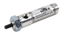
NITRA pneumatic cylinder, non-repairable, 3/4in bore, 1/4in rod diameter, 1/2in stroke, double acting, front nose mount.
