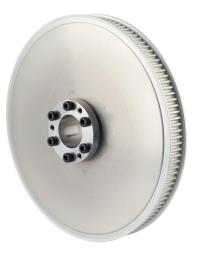
Sung-Il Machinery timing pulley, aluminum, 5mm 5M pitch, 120 tooth, 7.519in pitch diameter, 1-1/8in bore, no hub with flanges. For use with 15mm wide belt. QD bushing included.
