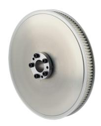
Sung-Il Machinery timing pulley, aluminum, 5mm 5M pitch, 120 tooth, 7.519in pitch diameter, 7/8in bore, no hub with flanges. For use with 15mm wide belt. QD bushing included.
