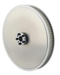
Sung-Il Machinery timing pulley, aluminum, 5mm 5M pitch, 120 tooth, 7.519in pitch diameter, 5/8in bore, no hub with flanges. For use with 15mm wide belt. QD bushing included.
