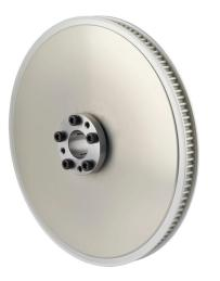
Sung-Il Machinery timing pulley, aluminum, 5mm 5M pitch, 120 tooth, 7.519in pitch diameter, 7/8in bore, no hub with flanges. For use with 9mm wide belt. QD bushing included.
