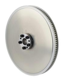
Sung-II Machinery timing pulley, aluminum, 5mm 5M pitch, 120 tooth, 7.519in pitch diameter, 3/4in bore, no hub with flanges. For use with 9mm wide belt. QD bushing included.
