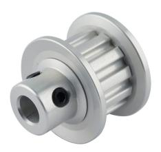
Sung-II Machinery timing pulley, aluminum, 1/5in XL pitch, 12 tooth, 0.764in pitch diameter, 1/4in bore, hub with flanges. For use with 3/8in wide belt.
