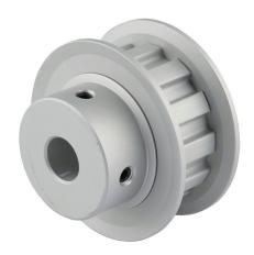
Sung-Il Machinery timing pulley, aluminum, 3/8in L pitch, 12 tooth, 1.432in pitch diameter, 3/8in bore, hub with flanges. For use with 1/2in wide belt.
