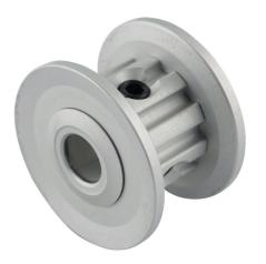
Sung-Il Machinery timing pulley, aluminum, 1/5in XL pitch, 10 tooth, 0.637in pitch diameter, 1/4in bore, no hub with flanges. For use with 3/8in wide belt.
