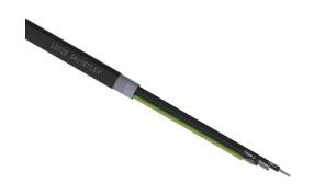
LUTZE DRIVEFLEX VFD cable, 4 conductors (includes ground), 18 AWG, 19-stranded, tinned copper, XLPE conductor insulation material, XHHW-2 jacket, black, cut to length.
