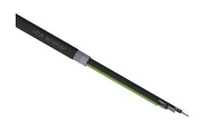
LUTZE DRIVEFLEX VFD cable, 4 conductors (includes ground), 16 AWG, 26-stranded, tinned copper, XLPE conductor insulation material, XHHW-2 jacket, black, cut to length.
