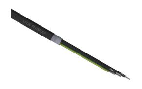
LUTZE DRIVEFLEX VFD cable, 4 conductors (includes ground), 14 AWG, 41-stranded, tinned copper, XLPE conductor insulation material, XHHW-2 jacket, black, cut to length.
