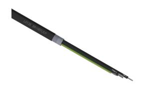
LUTZE DRIVEFLEX VFD cable, 4 conductors (includes ground), 14 AWG, 41-stranded, tinned copper, XLPE conductor insulation material, XHHW-2 jacket, black, cut to length.
