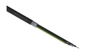
LUTZE DRIVEFLEX VFD cable, 4 conductors (includes ground), 12 AWG, 65-stranded, tinned copper, XLPE conductor insulation material, XHHW-2 jacket, black, cut to length.
