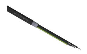
LUTZE DRIVEFLEX VFD cable, 4 conductors (includes ground), 10 AWG, 105-stranded, tinned copper, XLPE conductor insulation material, XHHW-2 jacket, black, cut to length.
