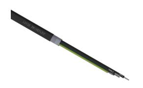
LUTZE DRIVEFLEX VFD cable, 4 conductors (includes ground), 8 AWG, 168-stranded, tinned copper, XLPE conductor insulation material, XHHW-2 jacket, black, cut to length.
