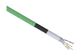
LUTZE flexible Cat6a industrial Ethernet Profinet cable, shielded, 4 twisted pairs, 22 AWG, solid, bare copper, special polyolefin conductor insulation material, PVC jacket, green, cut to length.
