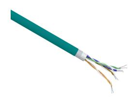
LUTZE flexible Cat5e industrial Ethernet cable, shielded, 4 twisted pairs, 22 AWG, 7-stranded, tinned copper, special polyolefin conductor insulation material, PVC jacket, teal, cut to length.
