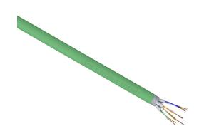
LUTZE flexible Cat6a industrial Ethernet cable, shielded, 4 twisted pairs, 26 AWG, 7-stranded, bare copper, special polyolefin conductor insulation material, PVC jacket, green, cut to length.
