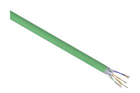
LUTZE flexible Cat6a industrial Ethernet cable, shielded, 4 twisted pairs, 26 AWG, 7-stranded, bare copper, special polyolefin conductor insulation material, PVC jacket, green, cut to length.
