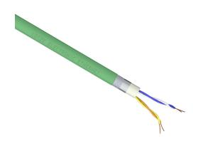
LUTZE flexible Cat5e industrial Ethernet cable, shielded, 2 twisted pairs, 22 AWG, 7-stranded, tinned copper, special polyolefin conductor insulation material, PVC jacket, green, cut to length.
