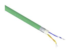
LUTZE flexible Cat5e industrial Ethernet cable, shielded, 2 twisted pairs, 22 AWG, solid, bare copper, special polyolefin conductor insulation material, PVC jacket, green, cut to length.
