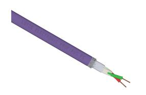
LUTZE Profibus cable, shielded, 1 twisted pair, 22 AWG, solid, bare copper, special polyolefin conductor insulation material, PVC jacket, purple, cut to length.
