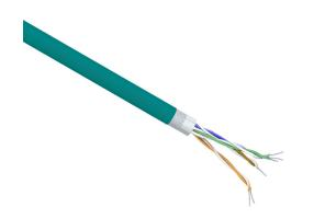
LUTZE MOTIONFLEX continuous flexing Cat6a industrial Ethernet cable, shielded, 4 twisted pairs, 24 AWG, 7-stranded, tinned copper, HDPE conductor insulation material, TPE jacket, teal, cut to length.
