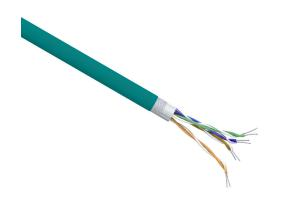
LUTZE MOTIONFLEX continuous flexing Cat5e industrial Ethernet cable, shielded, 4 twisted pairs, 24 AWG, 7-stranded, tinned copper, HDPE conductor insulation material, TPE jacket, teal, cut to length.
