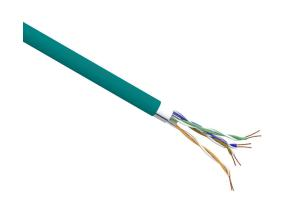
LUTZE Cat6 industrial Ethernet cable, shielded, 4 twisted pairs, 22 AWG, solid, bare copper, HDPE conductor insulation material, PVC jacket, teal, cut to length.
