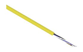
LUTZE IO-Link flexible control cable, unshielded, 5 conductors, 22 AWG, bare copper, PVC/Nylon conductor insulation material, black, brown, blue, white and gray, PVC jacket, yellow, cut to length.
