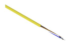
LUTZE IO-Link flexible control cable, unshielded, 4 conductors, 22 AWG, bare copper, PVC/Nylon conductor insulation material, black, brown, blue and white, PVC jacket, yellow, cut to length.
