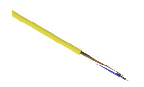
LUTZE IO-Link flexible control cable, unshielded, 4 conductors, 20 AWG, bare copper, PVC/Nylon conductor insulation material, black, brown, blue and white, PVC jacket, yellow, cut to length.
