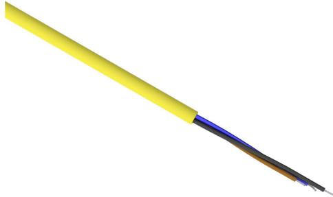
LUTZE IO-Link flexible control cable, unshielded, 3 conductors, 20 AWG, bare copper, PVC/Nylon conductor insulation material, black, brown and blue, PVC jacket, yellow, cut to length.
