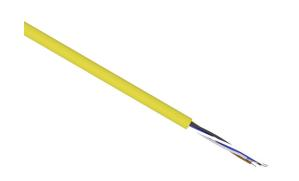
LUTZE IO-Link flexible control cable, unshielded, 5 conductors, 18 AWG, bare copper, PVC/Nylon conductor insulation material, black, brown, blue, white and gray, PVC jacket, yellow, cut to length.
