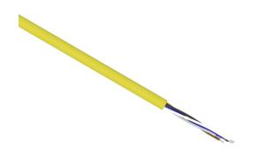
LUTZE IO-Link flexible control cable, unshielded, 5 conductors, 18 AWG, bare copper, PVC/Nylon conductor insulation material, black, brown, blue, white and gray, PVC jacket, yellow, cut to length.
