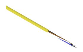
LUTZE IO-Link flexible control cable, unshielded, 4 conductors, 18 AWG, bare copper, PVC/Nylon conductor insulation material, black, brown, blue and white, PVC jacket, yellow, cut to length.
