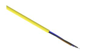
LUTZE IO-Link flexible control cable, unshielded, 3 conductors, 18 AWG, bare copper, PVC/Nylon conductor insulation material, black, brown and blue, PVC jacket, yellow, cut to length.
