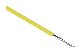
LUTZE IO-Link flexible control cable, unshielded, 5 conductors, 16 AWG, bare copper, PVC/Nylon conductor insulation material, black, brown, blue, white and gray, PVC jacket, yellow, cut to length.
