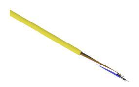
LUTZE IO-Link flexible control cable, unshielded, 4 conductors, 16 AWG, bare copper, PVC/Nylon conductor insulation material, black, brown, blue and white, PVC jacket, yellow, cut to length.
