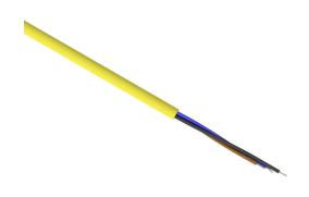
LUTZE IO-Link flexible control cable, unshielded, 3 conductors, 16 AWG, bare copper, PVC/Nylon conductor insulation material, black, brown and blue, PVC jacket, yellow, cut to length.
