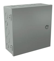
Wiegmann enclosure, NEMA 1, 10 x 10 x 4in (HxWxD), wall mount, with knockouts, carbon steel, ANSI 61 gray, powder coat finish, single-door, integral snap-tight latch.
