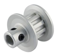
Sung-II Machinery timing pulley, aluminum, 1/5in XL pitch, 10 tooth, 0.637in pitch diameter, 1/4in bore, hub with flanges. For use with 3/8in wide belt.
