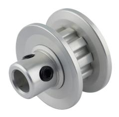
Sung-II Machinery timing pulley, aluminum, 1/5in XL pitch, 10 tooth, 0.637in pitch diameter, 1/4in bore, hub with flanges. For use with 1/4in wide belt.
