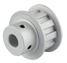
Sung-Il Machinery timing pulley, aluminum, 3/8in L pitch, 10 tooth, 1.194in pitch diameter, 3/8in bore, hub with flanges. For use with 1/2in wide belt.
