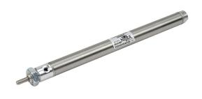
NITRA pneumatic cylinder, non-repairable, 9/16in bore, 3/16in rod diameter, 6in stroke, double acting, front nose mount.
