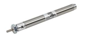
NITRA pneumatic cylinder, non-repairable, 9/16in bore, 3/16in rod diameter, 4in stroke, double acting, front nose mount.
