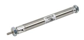
NITRA pneumatic cylinder, non-repairable, 9/16in bore, 3/16in rod diameter, 4in stroke, double acting, double end mount.
