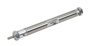
NITRA pneumatic cylinder, non-repairable, 9/16in bore, 3/16in rod diameter, 4in stroke, double acting, magnetic piston, double end mount.
