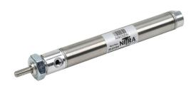
NITRA pneumatic cylinder, non-repairable, 9/16in bore, 3/16in rod diameter, 3in stroke, double acting, front nose mount.
