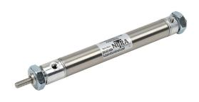
NITRA pneumatic cylinder, non-repairable, 9/16in bore, 3/16in rod diameter, 3in stroke, double acting, double end mount.
